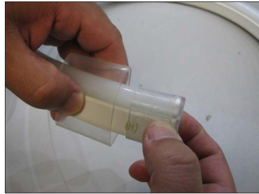
Shrink tubing the end cap
