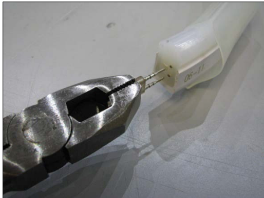
Blunt nose pliers holding power pin (Note: conductors toward right)
