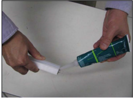
4.2 Apply 100% silicone around all power pins prior to assembly
