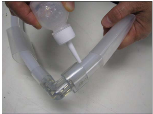
4.4 PVC glue edges of connectors
