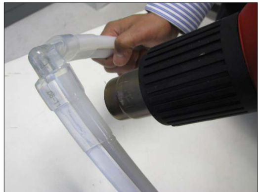
4.6 Cover all connection points with Heat Shrink Tubing and apply heat to seal all joints
