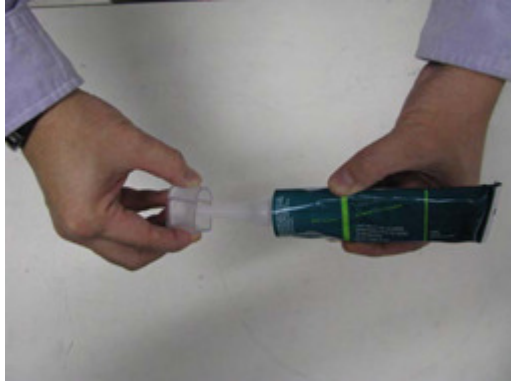
End cap with 100% silicone sealant
