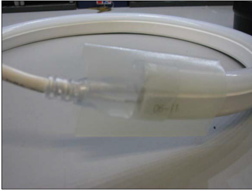
Position Shrink Tubing over power cord
