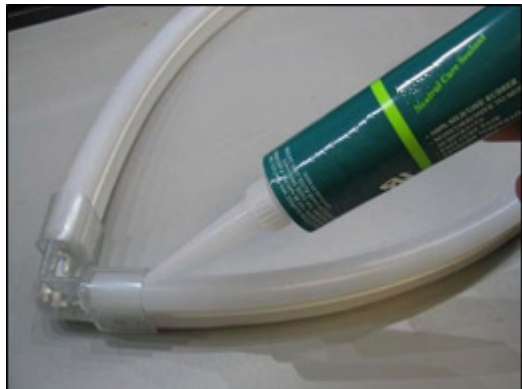
4.5 Use 100% silicone sealant to seal all connection points
