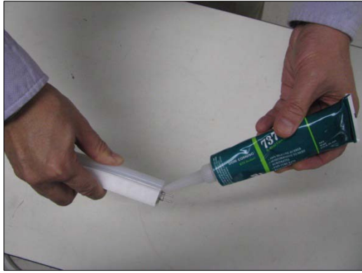
Apply Silicone around power pin 100% silicone sealant
