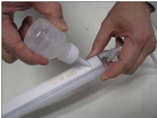
PVC glue around power cord shell
