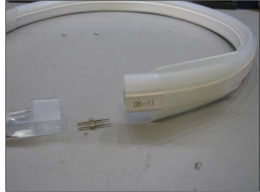
Heat Shrink tubing over power cord end
